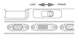
Figure 4-14. Locking the Port Replicator
